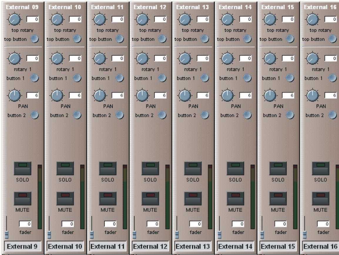
MIDI Messages are defined by touching the relevant on screen control and entering a MIDI channel, a command type and values for the parameters. At the bottom of the panel a MIDI port can be selected - Port A represents the first COMBI card, B is the second COMBI card and T is the standard built in MIDI port on the console.
