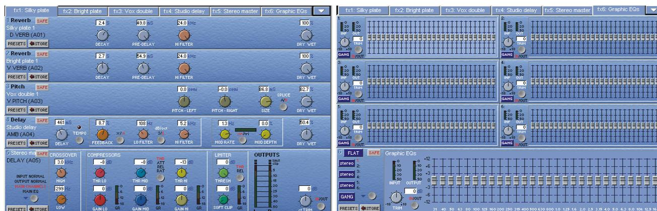
Graphics EQ's can be ganged with relative offsets by pressing the relevant on screen **Gang** buttons and individual faders can be reset using the worksurface master solo buttons.
